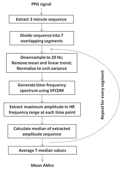
Fig 2. Processing steps for calculating the amplitude estimates in the HR frequency range.
