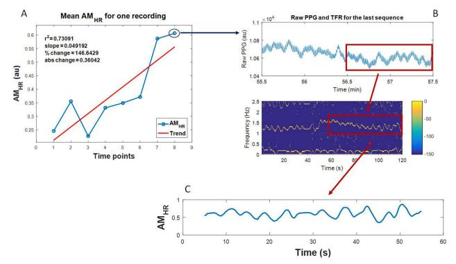
Fig 3. An illustrative example of a calculated feature vector for one trauma patient's recording. A: The plot of mean  $AM_{HR}$  values at various time points, the trend line, and the corresponding features. B: The plot of the raw PPG and the corresponding VFCDM TFR of the 2 minute sequence at the last time point (point 8). C: Sequence of  $AM_{HR}$  values extracted from the last 1 minute TFR.
