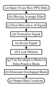
Figure 2. Flowchart of the WEPD algorithm.
